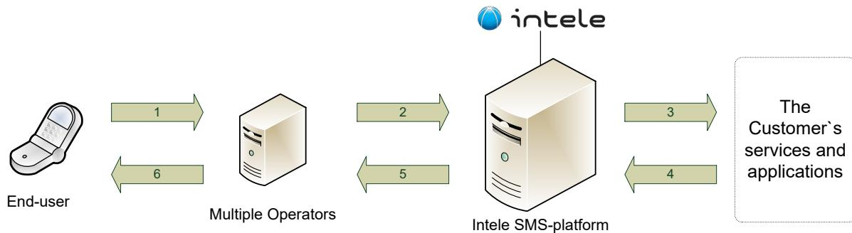
The figure above provides an overview of the traffic flow between the End-user and the Customer. The message flow can be initiated both by the End-user (Mobile Originating) and by the Customer (Mobile Terminating).
